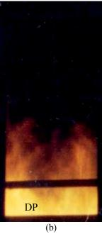
Zone of turbulent mixing on interface: a detonation products (DP) of mixture of acetylene with oxygen - air (Air) in experiments on the shock tube working under the method [2] a) Shadow black-and-white photo of a zone of mixing and b) a color photo of own luminescence of products of a detonation
