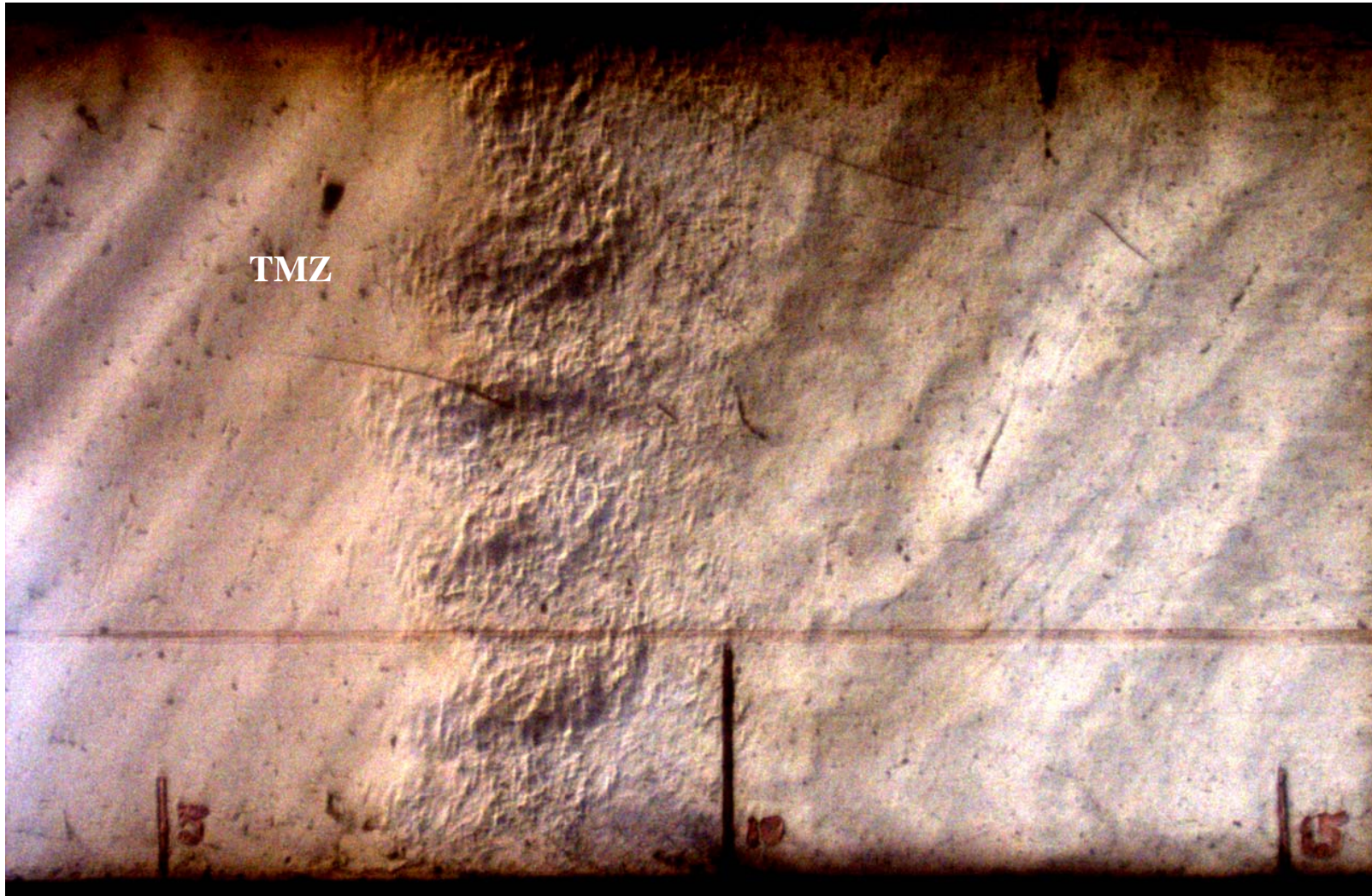
Fig.4. Picture of current in a shock tube (fig.2) at the moment of time t=700 mks (after passing through interface shock wave reflected from rigid wall 2). Designations: TMZ - a turbulent mixing zone on interface between products of a detonation and air.
