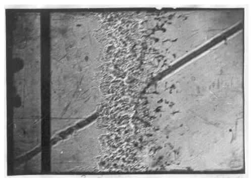
Photo of *turbulent mixing* zone on air - helium interface in experiments such as [1], received by a *Ronchi* method at the moment of time t=890 mkc after the beginning of movement of interface. Designations: TMZ-zone TII; F-.shadow of string, size of a defocusing  $\Delta = 210$  mm,
