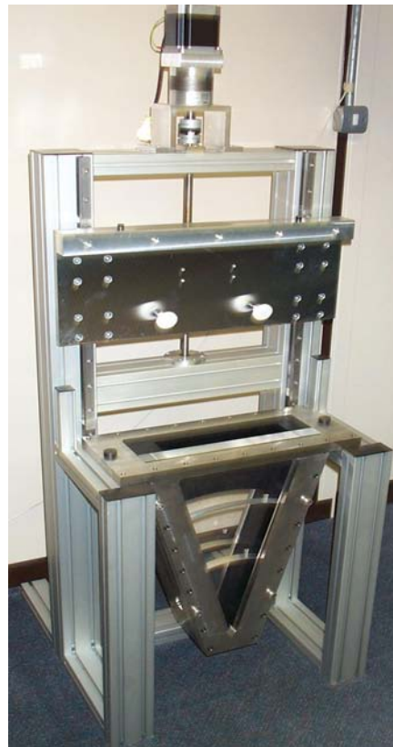
Figure 12. CST support stand with test cell and frame in place.
