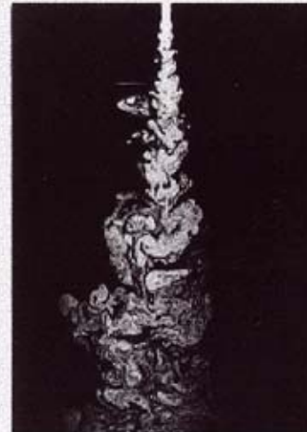
Liquid-jet concentration in a round turbulent jet (Dimotakis 1983)
