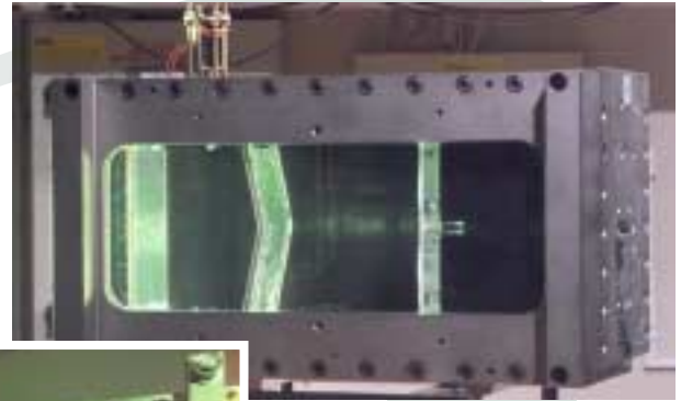
Test Cell Chevron Interface Profile SF_6 gives Atwood Number, A=0.67
