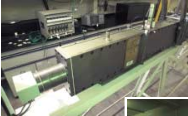
Compression Chamber Pressurised with Air to 2 bar
