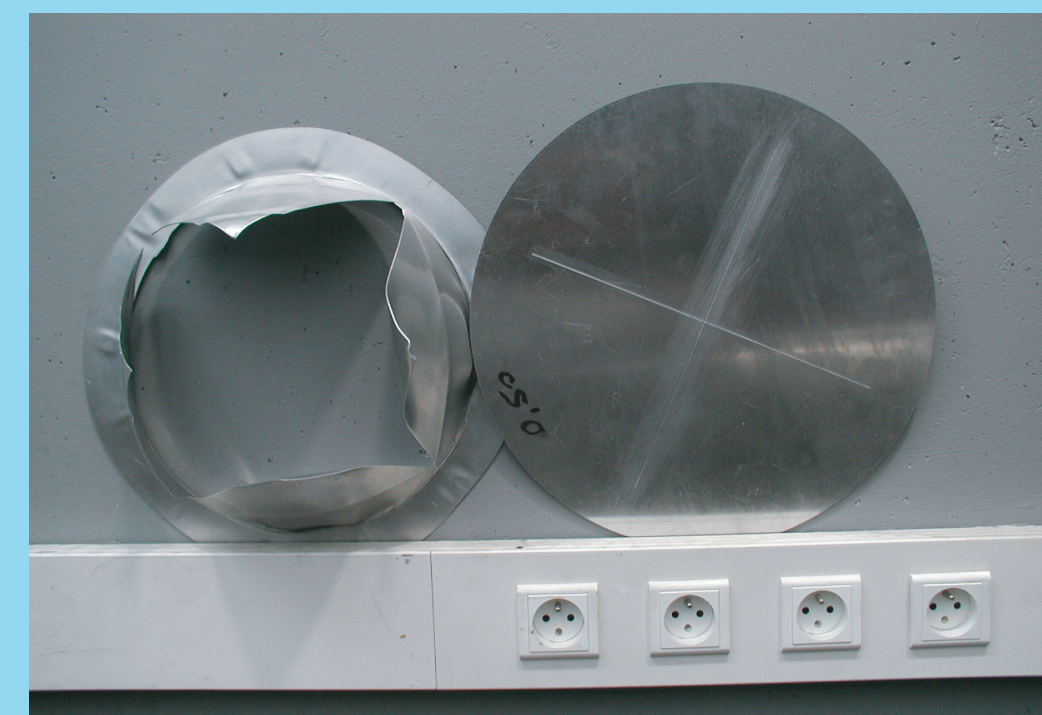
First diaphragm before and after run (Aluminium, thickness=1 mm, φ=360 mm)
