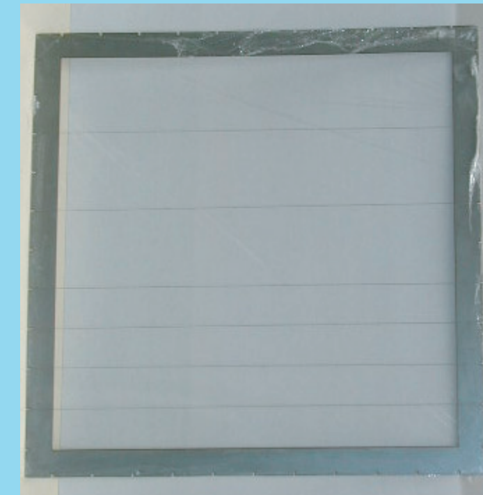
Initial interface materialized by a 0.8 μm thick nitrocellulose membrane resting over metallic horizontal lines
