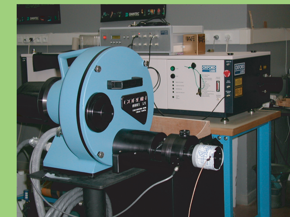
321 Cordin camera coupled with the LS 20-50 copper vapour Oxford laser
