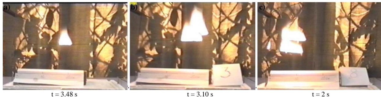
Figure 1. Flame propagation along a) a thread saturated with kerosene, b) two threads diverging from a point, c) two parallel threads
