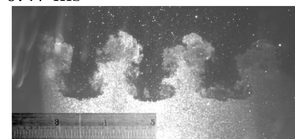
Experimental image at t=0.70 ms after shock interaction. Measured amplitude \eta=17.52 mm
