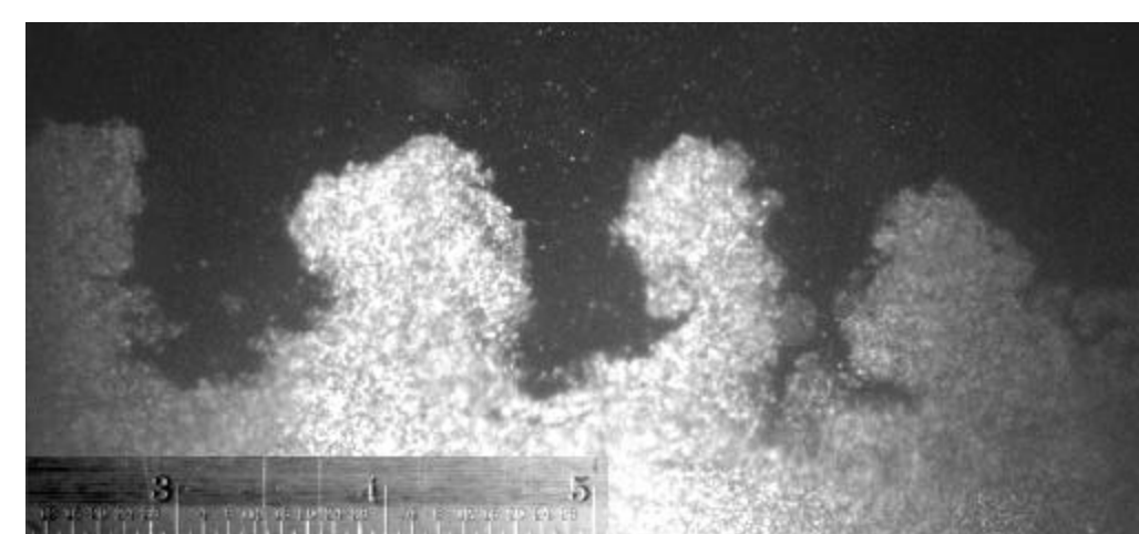
Experimental image at t=0.66 ms after shock interaction. Measured amplitude \eta=15.29 mm
