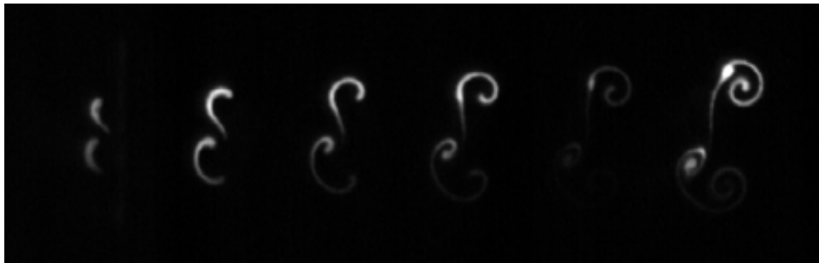
Figure 1. Flow visualization example of interaction between adjacent shock-accelerated gas cylinders.
