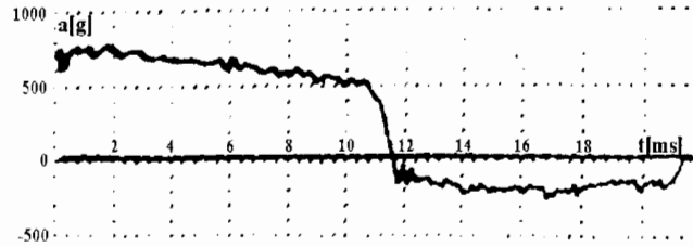
Figure 3. Characteristic oscillogram of the ampoule acceleration in experiments with n = 3 at S^* = 360 mm.
