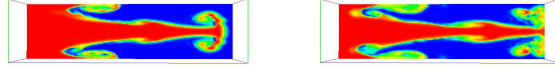
Figure 1: Section at x_2 = L_{x_2}/2 for t = 5.75ms (left) and t = 6.83ms (right) for a (2, 2) order calculation; the denser fluid (left) penetrates the less dense one by developing the well-known mushroom shape, secondary instabilities are observed at the interface.
