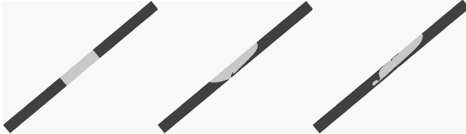
Fig. 3.1. Transition to steady-state rise. One finite bubble in the “infinitely” long pipe, \alpha = 45^\circ , \mu = 0.1
