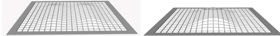
Fig. 4.5. Grid designs using the software CATIA (grid 1: \lambda_0=80\text{mm} - \eta_0 = 3\text{mm} , grid 2: \lambda_0=120\text{mm} - \eta_0 = 6\text{mm} ).
