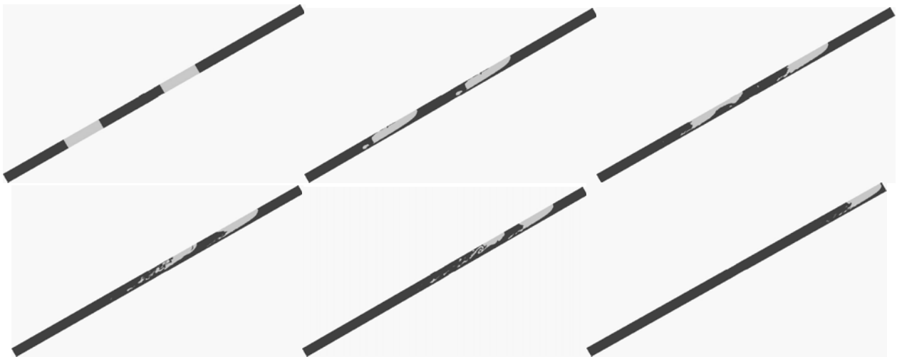
Fig. 3.2. Two bubbles in the long pipe, \alpha = 45^\circ . (1) Initial state, (2) non-interacting bubbles {non-interacting because the trace of the upper bubble is shorter than the liquid slug between the bubbles}, (3) the influence of the trace of the upper bubble on the lower bubble begins, (4,5) due to shear in the trace of the upper bubble the lower bubble rises faster than the upper bubble – the distance separating them decreases, (6) merging of two bubbles into one bubble
