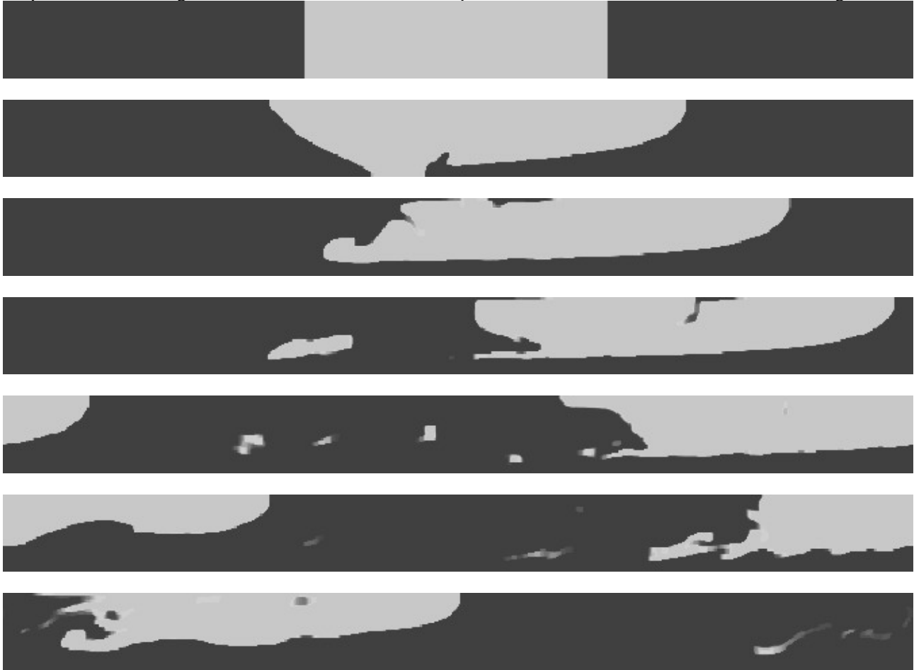
Fig. 3.3. Establishing of steady-state flow of the periodic slug chain, \alpha = 20^0 . Time increases from the upper to the lower frame
