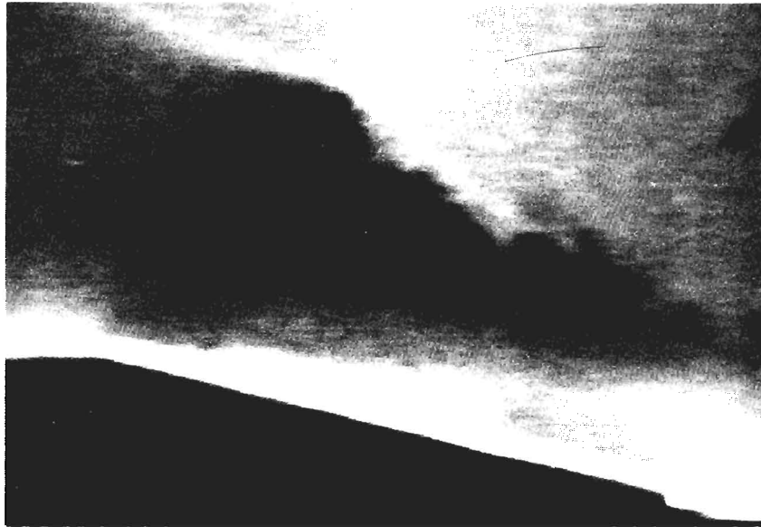
Figure 14. Shock wave/boundary layer interaction in a Mach 3 flow with a 16^\circ angle wedge.
