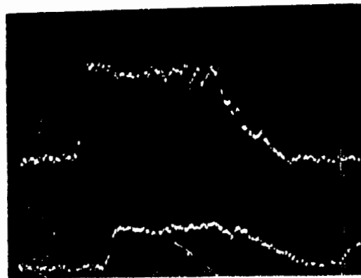
Figure 2 : Example of oscillographic emission records for CO_2/Ar mixing zone thickness determination.
